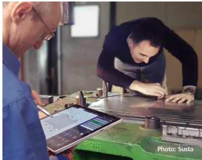
Die setup assessment using AutoForm-TryoutAssistant in a tool shop
