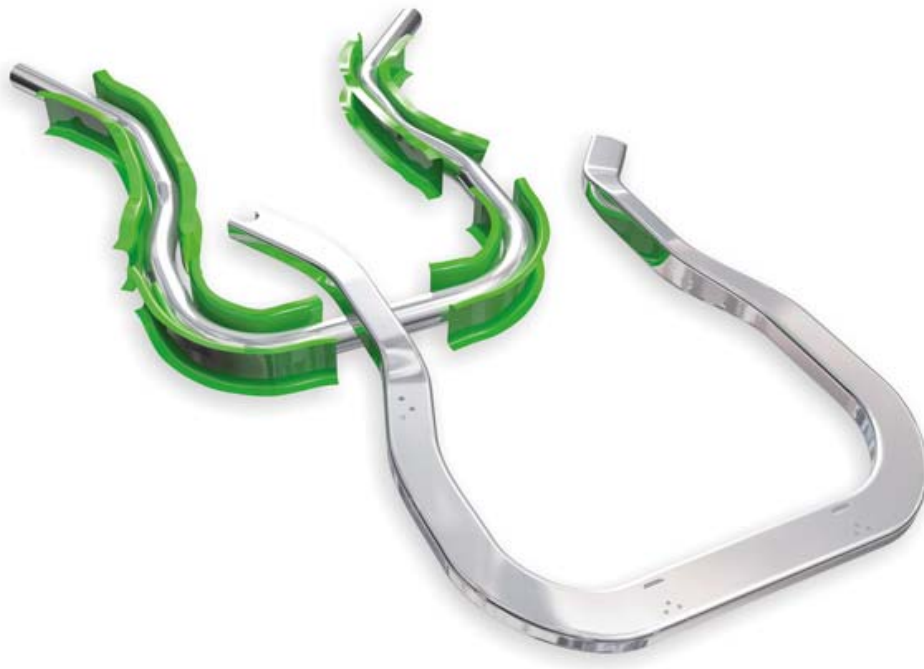
Hydroforming of engine cradle in high strength steel – preforming and final part.
